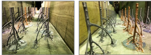
Fig 2. 3D-printed mangroves in the wave flume
