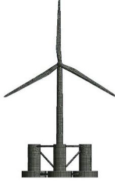
Fig. 4 Mesh discretization of the DeepCwind FOWT.
